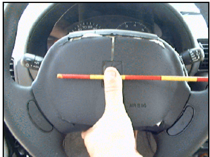
Figure 6. Interior, case vehicle. Driver's side air bag flaps.
