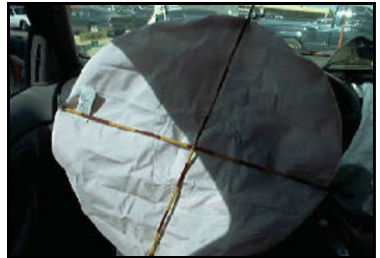
Figure 8. Deployed Drivers Air Bag
