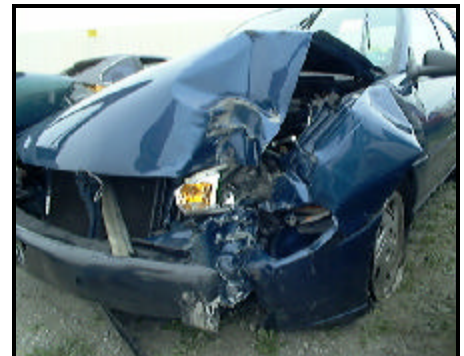
Figure 8. Primary impact to left corner (pole impact / Event #3)
