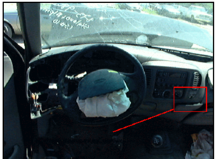
Figure 5. Interior, case vehicle. Box indicates location of air bag shut off switch.
