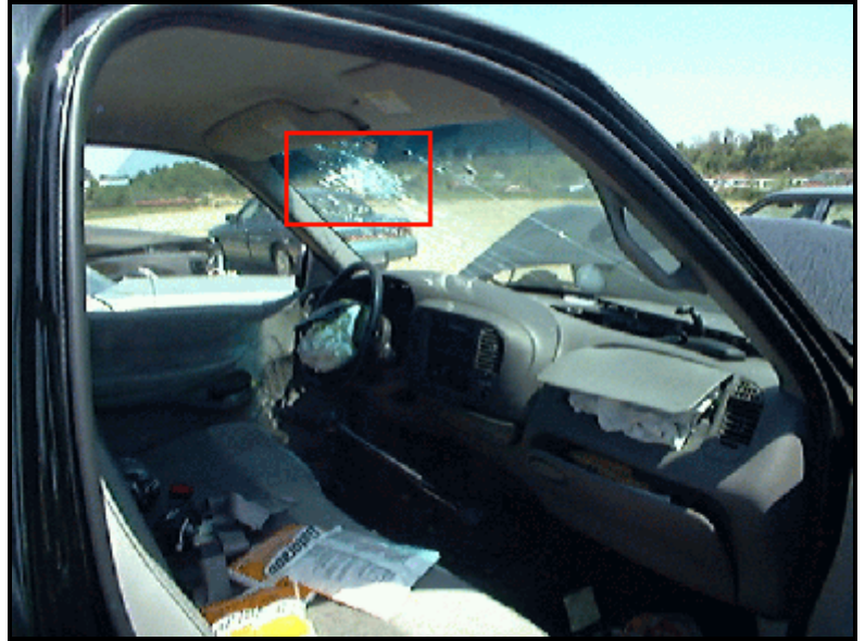
Figure 6. Interior, case vehicle. Box shows head contact.
