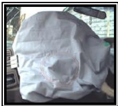
Figure 5. 1998 Chevrolet K-1500 pickup redesigned driver air bag.
