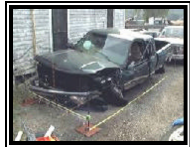
Figure 3. Frontal damage to the 1998 Chevrolet K-1500 pickup truck.
