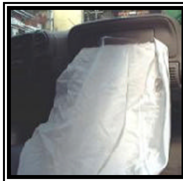
Figure 6. 1998 Chevrolet K-1500 pickup redesigned passenger air bag.
