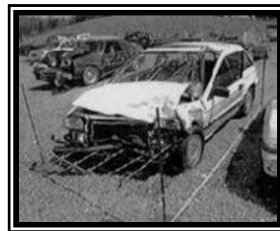
Figure 4. Front left damage to the 1986 Honda Civic.
