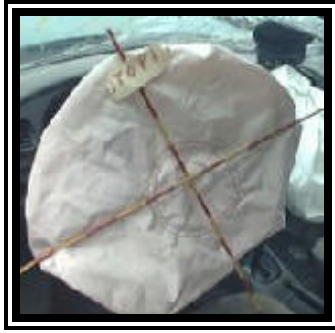
Figure 5. 1998 Ford Escort LX redesigned driver air bag.
