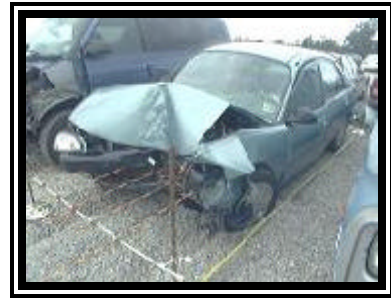
Figure 3. Frontal damage to the 1998 Ford Escort LX.
