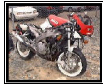
Figure 4. Frontal damage to the 1992 Yamaha FZR1000 motorcycle.
