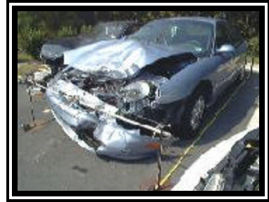
Figure 3. Frontal damage to the 1998 Ford Taurus SE.
