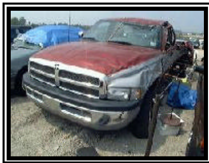
Figure 4. Top and left side surface damage to the 1997 Dodge Ram pickup truck.
