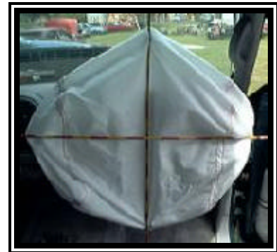
Figure 7. 1998 Chevrolet Suburban redesigned passenger air bag.
