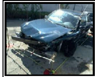
Figure 2. Front left damage to the 1998 Toyota Corolla.
