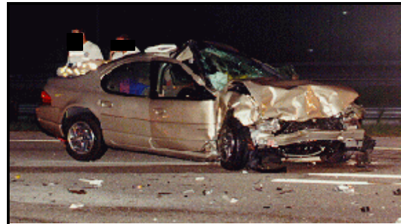
Figure 3: Case vehicle's front contact damage and induced damage on right side
