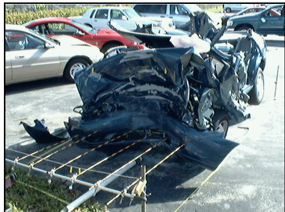
Figure 5: Front left view of damage measurement
