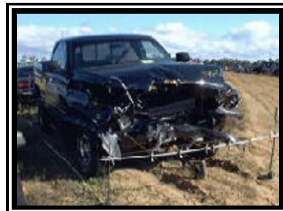
Figure 3. Frontal damage to the 1998 Dodge Ram pickup truck.
