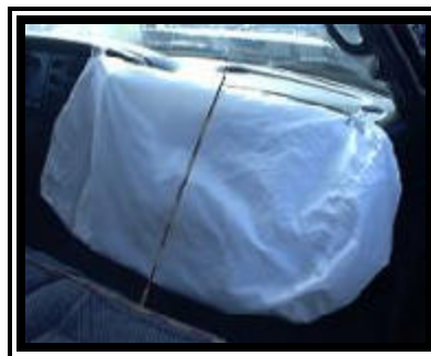
Figure 6. 1998 Dodge Ram redesigned passenger air bag.
