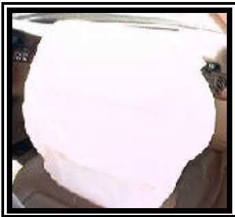
Figure 6. 1998 Cadillac Deville redesigned passenger air bag.
