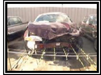
Figure 3. Frontal damage to the 1998 Dodge Stratus .
