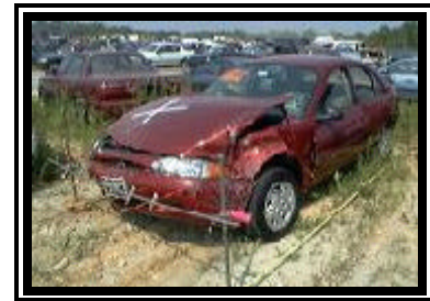
Figure 3. Frontal damage to the 1998 Ford Escort LX.
