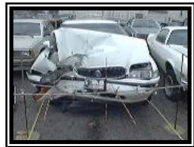
Figure 2. Frontal damage to the 1998 Buick LeSabre.
