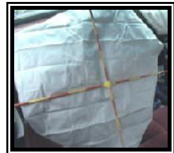
Figure 4. 1998 Buick LeSabre redesigned driver air bag.
