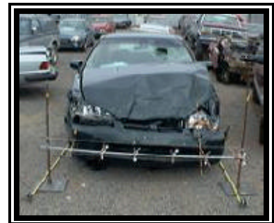
Figure 3. Frontal damage to the 1998 Honda Accord LX.
