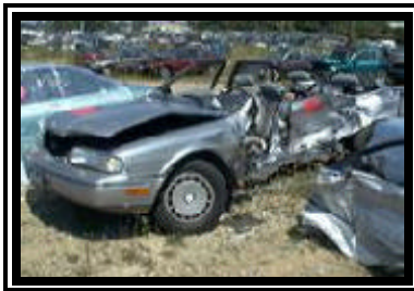
Figure 4. Left side damage to the 1990 Infinity Q45.
