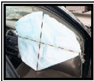
Figure 7. 1998 Honda Accord LX redesigned passenger air bag.
