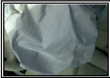
Figure 7 - View of the front left non-tethered air bag showing the striated transfer pattern from contact with the air bag module cover
