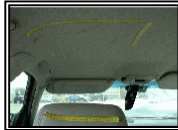
Figure 5 - View from rear seat looking forward of contact evidence on the roof head liner and rear surface of the driver seat head restraint
