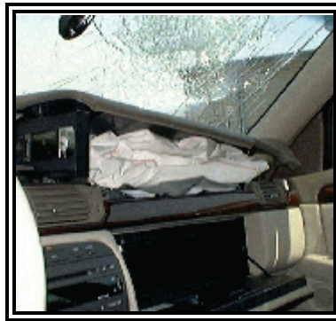
Figure 8 - View of the front right air bag relocated back under the instrument panel
