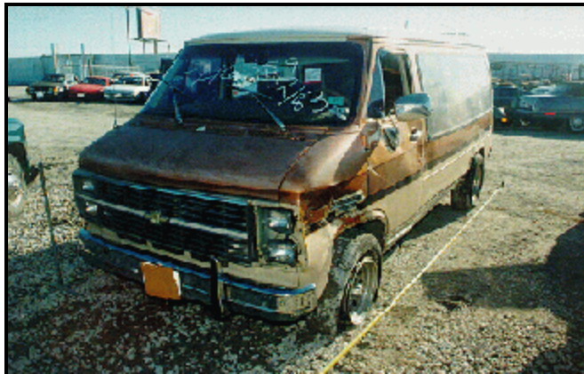
Figure 11: Vehicle #2 left side rollover damage (case photo #35)
