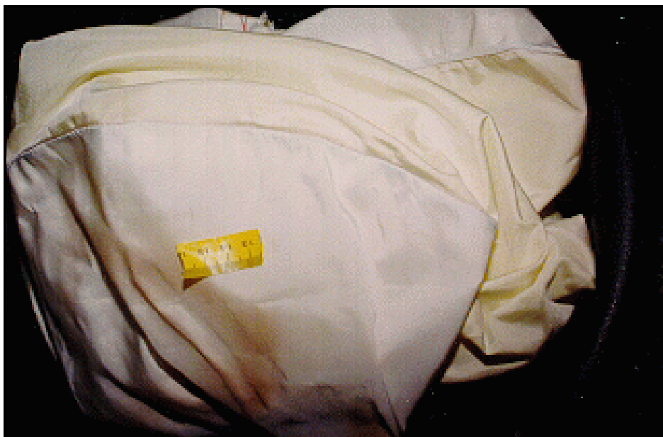
Figure 9: Back bottom half of case vehicle's driver's air bag -- tape indicates area of scorching (case photo #28)
