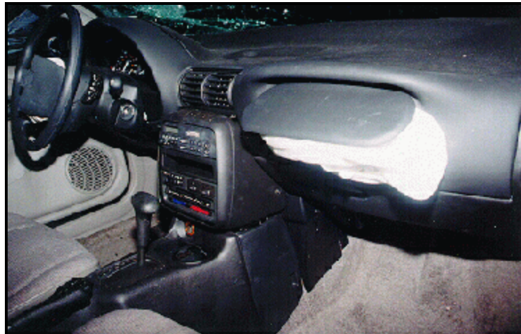
Figure 7: Case vehicle's front right air bag module (case photo #29)
