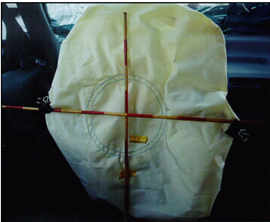
Figure 8: Front of case vehicle's driver air bag -- tape indicates area of scuffs and discoloration (case photo #25)
