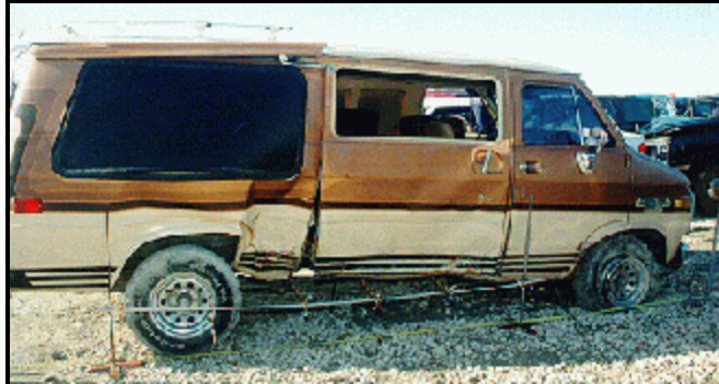
Figure 10: Vehicle #2 right side damage from impact with case vehicle (case photo #42)
