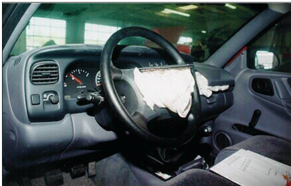
Figure 12: Case vehicle's front seating area showing deployed driver and front right passenger air bags and no contact evidence on steering wheel, left instrument panel, or driver's knee bolster (case photo #18)
