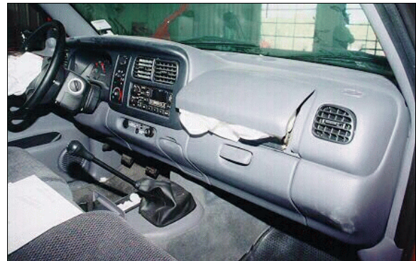
Figure 13: Case vehicle's deployed driver and front right passenger air bags and instrument panel areas; Note: no contact evidence on front right air bag module's cover flap or center or right instrument panel areas (case photo #27)
