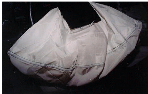
Figure 8: Case vehicle's deployed driver air bag showing no contact evidence on top/back surface of air bag or to air bag module's top cover flap (case photo #21)
