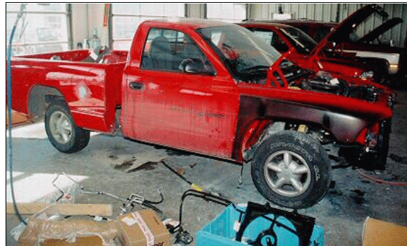
Figure 7: Case vehicle's right side showing repairs to right fender and right side of truck bed; Note: rightward shift to truck bed (case photo #12)
