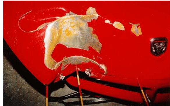
Figure 5: Close-up of narrow object impact to right side of case vehicle’s hood (case photo #15)
