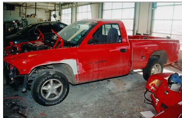
Figure 6: Case vehicle’s left side showing repairs to left fender and edge of left front door; Note: induced damage to truck bed (case photo #09)
