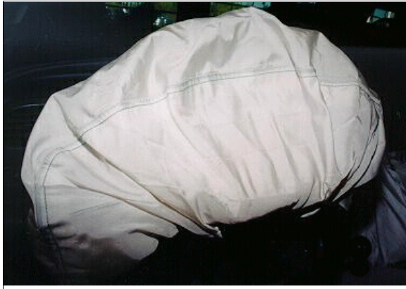
Figure 10: Case vehicle's deployed driver air bag showing no contact evidence on bottom/back surface of air bag (case photo #25)
