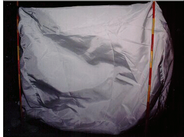
Figure 11: Case vehicle's deployed front right passenger air bag showing no contact evidence on air bag's front surface (case photo #30)
