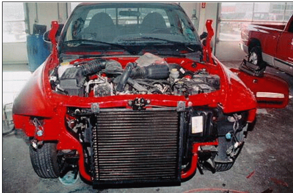
Figure 3: Case vehicle's partially repaired frontal damage; Note: new radiator and damaged hood along left side of vehicle (case photo #07)
