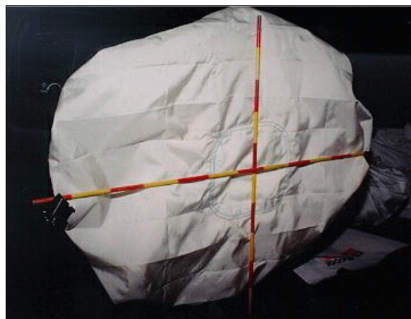
Figure 9: Case vehicle's deployed driver air bag showing no contact evidence on air bag's front surface (case photo #22)
