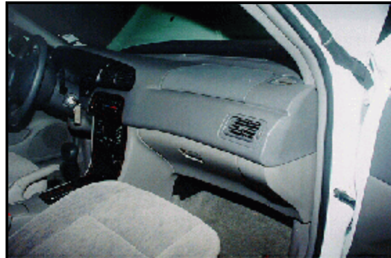
Figure 8: Case vehicle's front seating area showing location of deployed driver and front right passenger air bag modules; Note: replacement modules have been installed (case photo #17)
