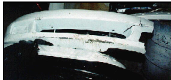
Figure 4: Case vehicle's damaged front bumper cover; Note: scrapes on bottom of bumper (case photo #10)
