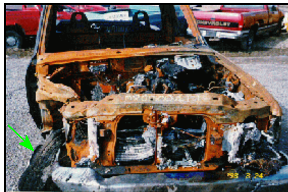
Figure 1: Case vehicle's frontal damage; Note: position of right front tire and right fender damage (case photo #01)
