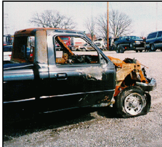
Figure 2: Case vehicle's front right damage; Note: direct damage to right front wheel rim and minimal fire damage to right front door (case photo #05)
