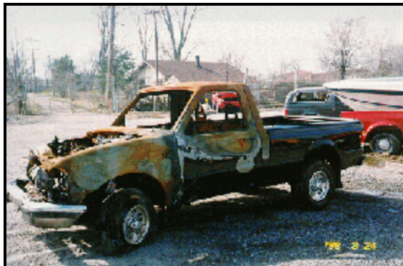
Figure 3: Case vehicle's fire damage; Note: paint on truck bed has only minor damage (case photo #02)
