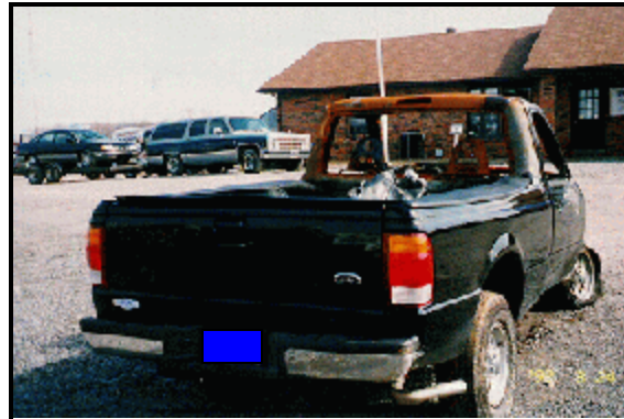
Figure 8: Case vehicle's back and right side; Note: backlite glazing gone and undamaged truck bed (case photo #04)
