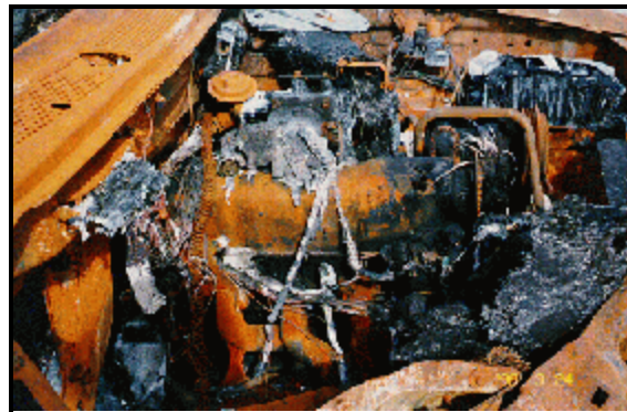
Figure 4: Fire damage to case vehicle's engine compartment, viewed from right side (case photo #06)
