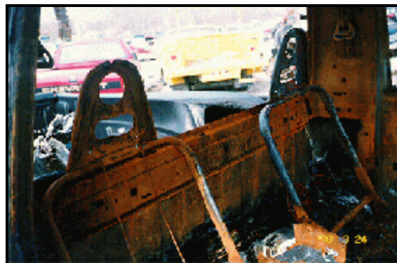
Figure 7: Fire damage to case vehicle's front seats; Note: integral head restraint frames and adjustable shoulder belt anchorage (case photo #08)
