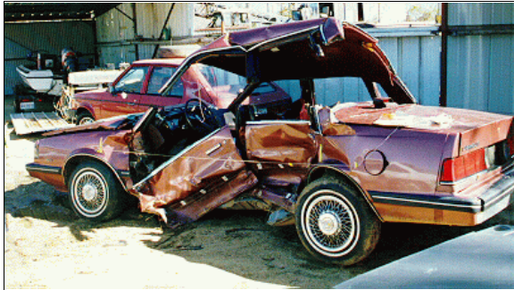
Figure 6: Chevrolet's left side damage (case photo #56)
