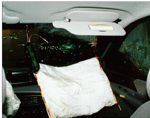
Figure 8: Contacts to case vehicle's front right windshield (i.e., spider web with hair) and header/sun visor; in addition, there were blood spots on upper left side of front right air bag (case photo #29)
