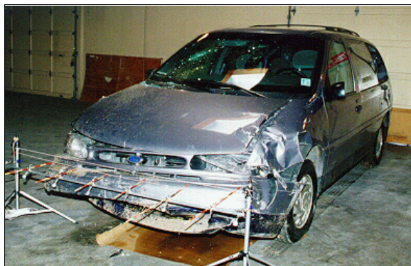
Figure 4: Case vehicle's frontal damage viewed from left of front with contour gauge present (case photo #15)
