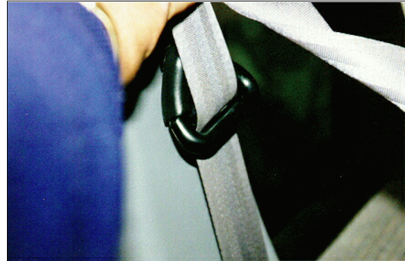
Figure 21: Case vehicle’s driver safety belt showing heat abrasion to “D”-ring (case photo #50)
