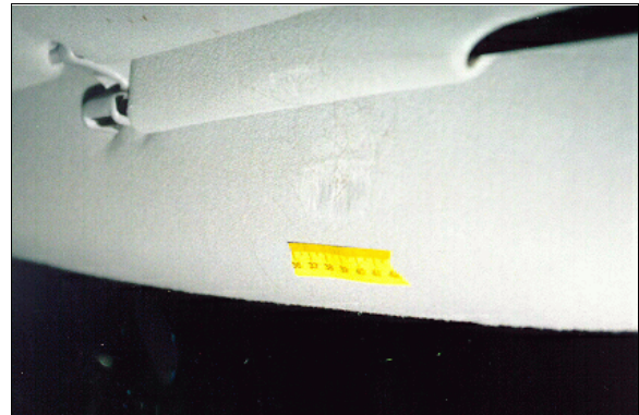
Figure 10: Close-up of case vehicle’s front right header showing evidence (i.e., hair, scuff) of contact (case photo #32b)
