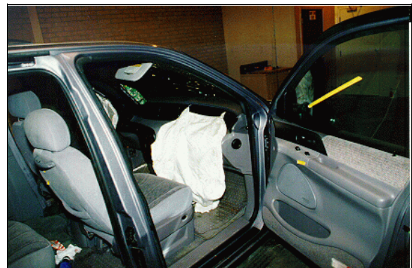
Figure 12: Case vehicle’s front right seating area and interior view of right front door showing deployed front right air bag and oil smear (i.e., yellow tape) to right front door’s glazing from contact by “on-lap” front right passenger (case photo #33)
