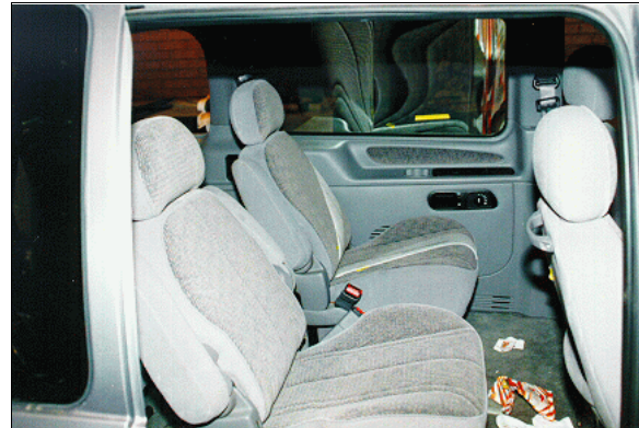
Figure 14: Case vehicle's second seating area; Note: contact to glazing by second seat left passenger (case photo #46)
