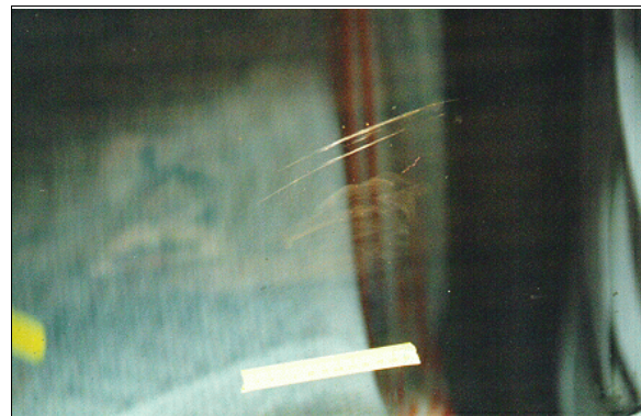
Figure 16: Close-up of make-up and oil smear on interior of left glazing for case vehicle's second seating area (case photo #51)
