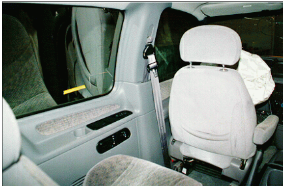
Figure 15: Seating area of case vehicle's second seat left passenger showing contact to side glazing; Note: driver's safety belt, box-mounted seat, and deployed air bag (case photo #49)
