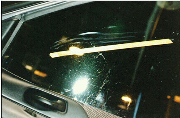
Figure 13: Close-up interior view of case vehicle's right front door glazing showing oil smears and fluid on glazing (case photo #34)
