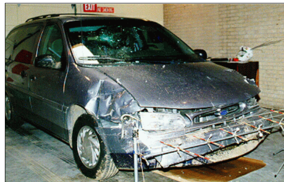
Figure 5: Case vehicle's frontal damage viewed from right of front with contour gauge present (case photo #21)
