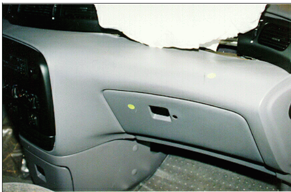
Figure 11: Case vehicle’s front right seating area showing scuffs to glove box door and a black scuff to top of dash (case photo #31)
