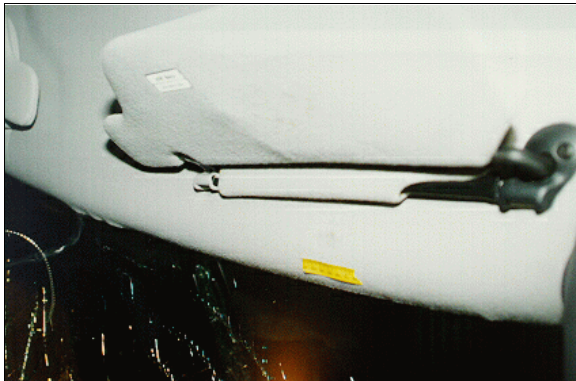
Figure 9: Case vehicle’s right sun visor (in raised position) and front right header showing occupant contact evidence on header (case photo #32a)
