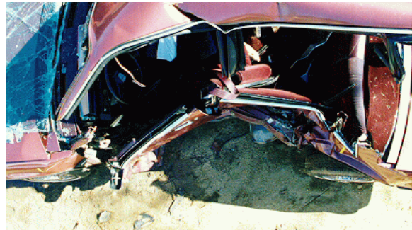
Figure 7: Overhead view of crush to Chevrolet's left side showing extensive intrusion into driver's space (case photo #57)
