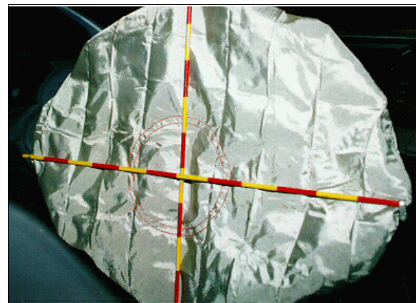
Figure 17: Case vehicle's deployed driver air bag showing no visible contact evidence, but there was sprayed cola on right half (case photo #37)
