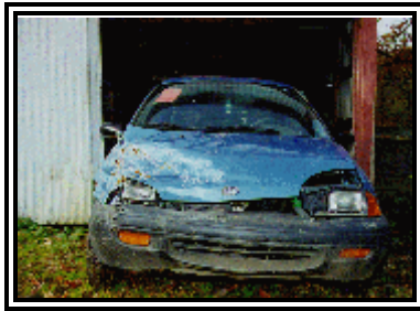
Figure 4. Frontal damage to the Geo Metro.
