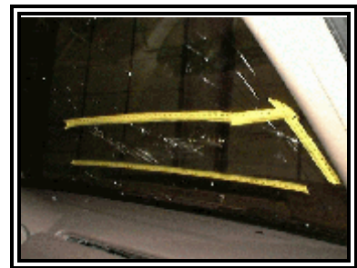
Figure 6: View of the right windshield fractures.
