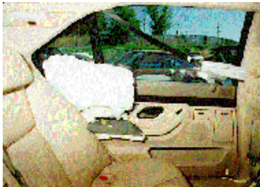
Figure 12. Deployed left rear door mounted side impact air bag.
