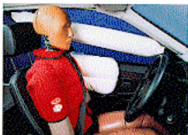
Figure 2. Test image of the deployed side impact air bags.
