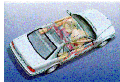
Figure 8. View of the BMW's frontal and side impact air bag systems.
