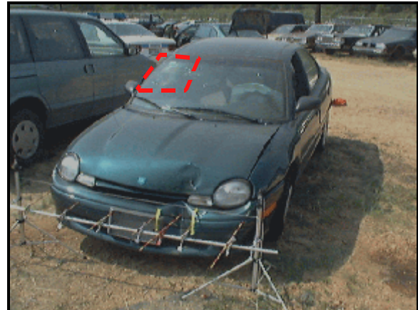
Figure 6: Overhead left view of case vehicle’s direct and induced frontal damage from pole impact; Note: windshield glazing on passenger side near header damaged from contact by “On-Lap” front right passenger’s head (case photo #13)
