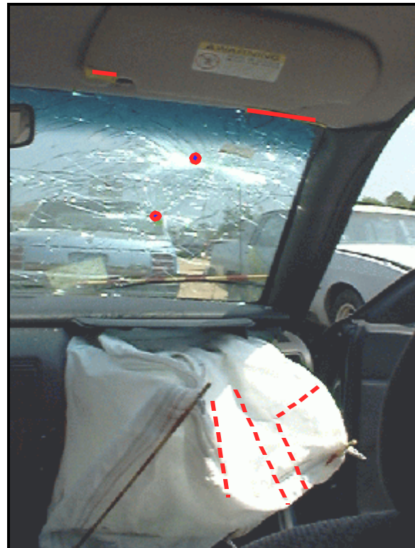
Figure 19: Vertical view of case vehicle's front right passenger seating area; Note: highlighted contacts to top of front right air bag, windshield, and right header (case photo #40)
