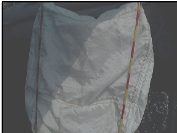
Figure 18: Frontal view of case vehicle's front right passenger air bag showing no visible evidence of contact (case photo #37)
