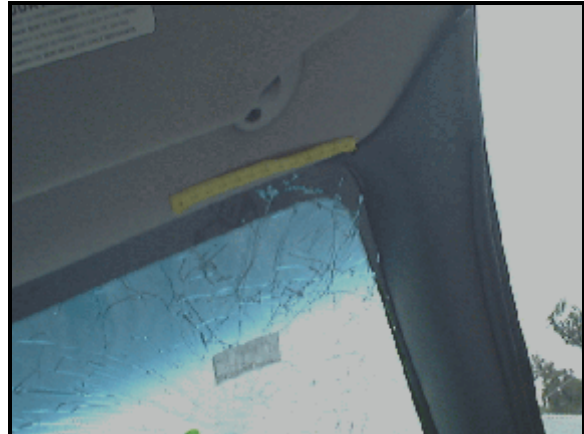
Figure 12: Close-up of head contact to case vehicle’s right upper windshield and header, near right “A”-pillar (i.e., hair and skin stuck in crease) from back of “On-Lap” front right passenger’s head (case photo #32)
