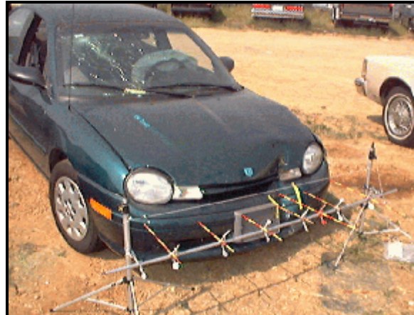
Figure 8: Overhead right view of case vehicle's front left damage with contour gauge present and tape indicating width of direct damage; Note: disintegrated right front door glazing and spider web type impacts to windshield (case photo #20)
