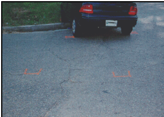
Figure 3: On-scene view showing police marked front tire skids of case vehicle at final rest; Note: curb impacted by left front wheel and vehicle's counterclockwise rotation to final rest position (case photo #47)
