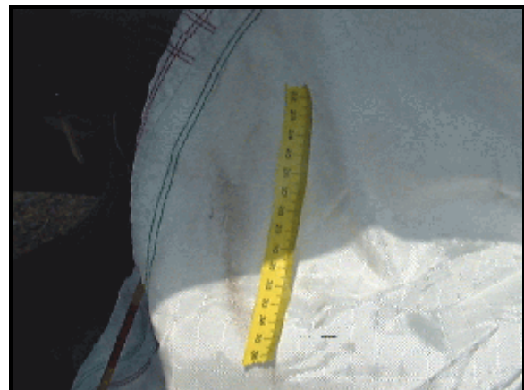
Figure 21: Dark skin transfer on right side near top front corner of case vehicle's front right passenger air bag (case photo #40)
