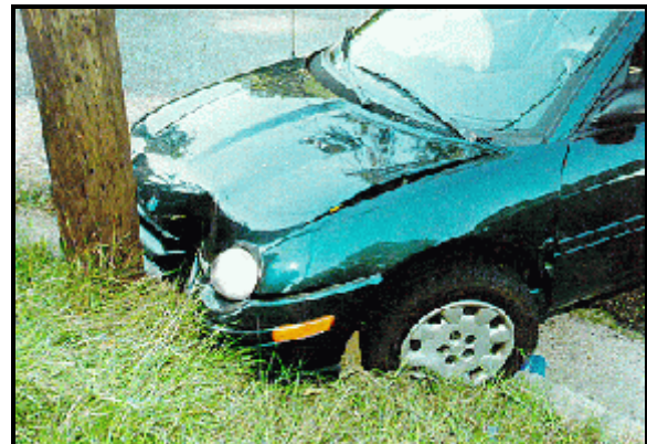
Figure 7: On-scene view of case vehicle at final rest; Note: case vehicle struck curb with the left front tire and wooden utility pole with front left (case photo #44)
