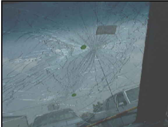
Figure 11: Close-up of spider web-type damage to case vehicle’s right upper windshield (upper dot) from impact by “On-Lap” front right passenger; Note: lower dot most likely represents contact by air bag’s fabric during deployment (case photo #31)
