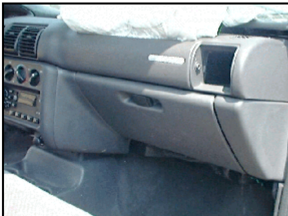
Figure 13: Case vehicle’s center and front right instrument panel, right knee bolster, and glove box door showing no evidence of occupant contact; Note: right air vent knocked out (case photo #30)
