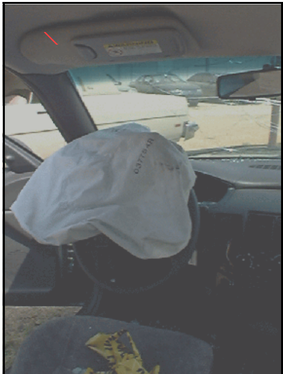
Figure 14: Vertical view of case vehicle’s driver seating area showing no visible contact evidence on driver’s air bag and a head contact (highlighted) to the left side of driver’s sun visor (case photo #25)
