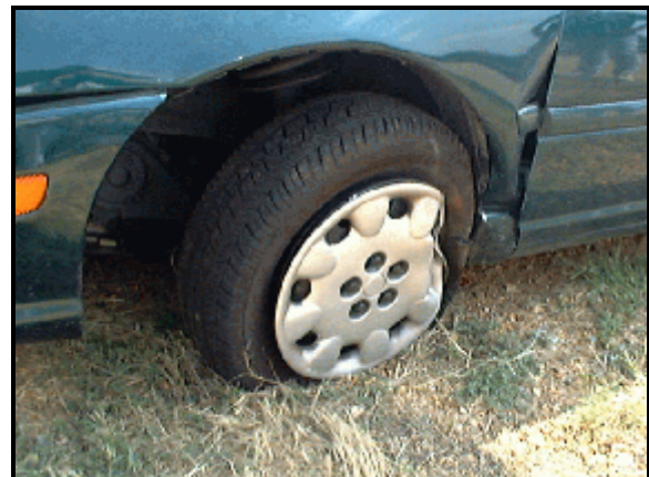
Figure 5: Damage to case vehicle's left front tire and wheel assembly from impacting curb (case photo #16)
