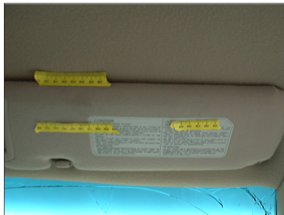
Figure 12: Close-up of case vehicle's right sun visor showing contact evidence from front right passenger's head (case photo #36)
