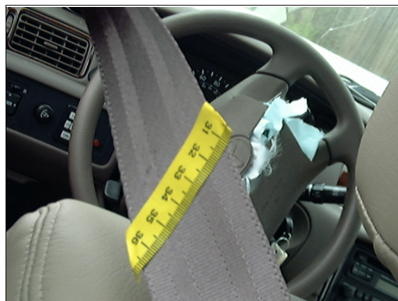
Figure 19: Close-up of loading evidence on case vehicle's driver safety belt (case photo #25)
