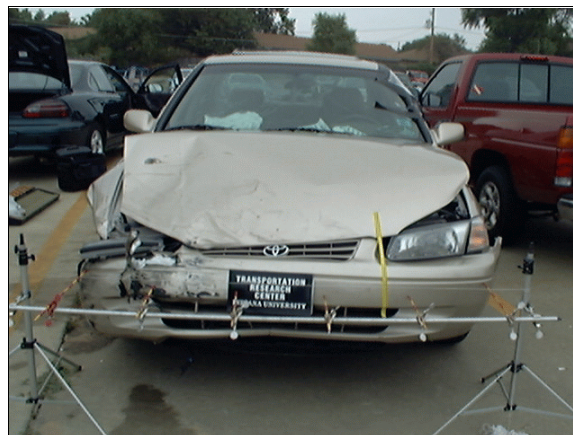
Figure 4: Case vehicle's frontal damage with contour gauge present; Note: direct damage extends along front from front right corner to yellow tape (case photo #16)
