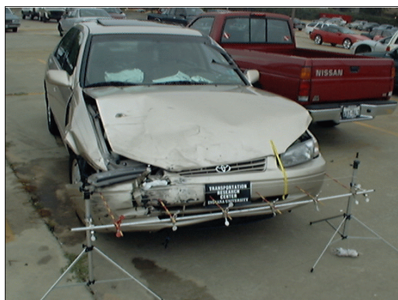
Figure 5: Case vehicle's damaged front viewed from right of front with contour gauge present; Note: yellow tape highlights end point of direct damage (case photo #09A)
