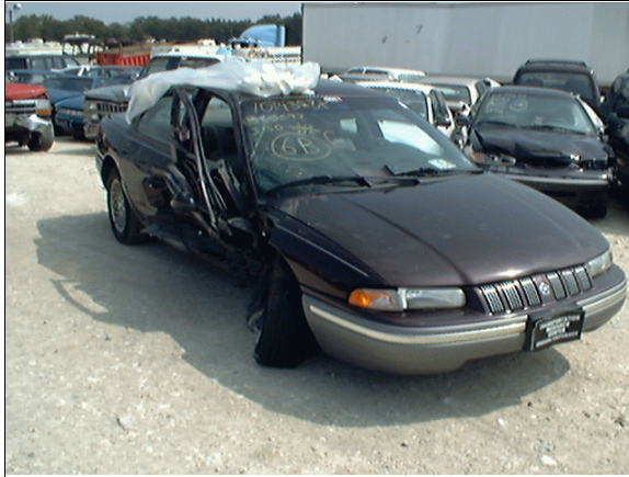
Figure 7: Chrysler's damaged right side viewed from right of front (case photo #63)
