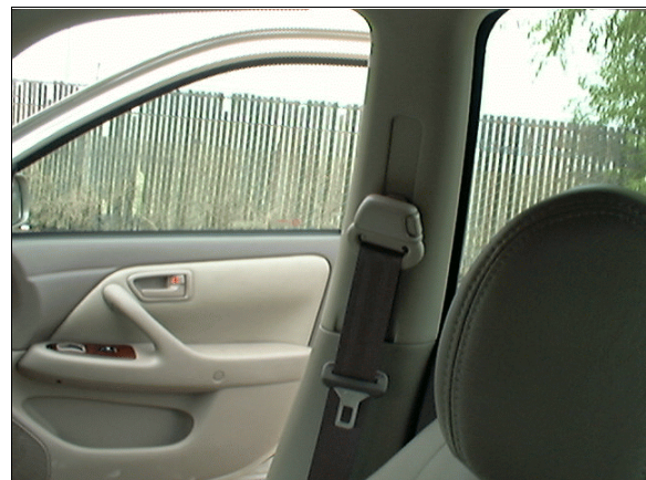
Figure 18: Case vehicle's unused front right passenger safety belt system; Note: adjustable upper anchorage located in down-most position (case photo #37)
