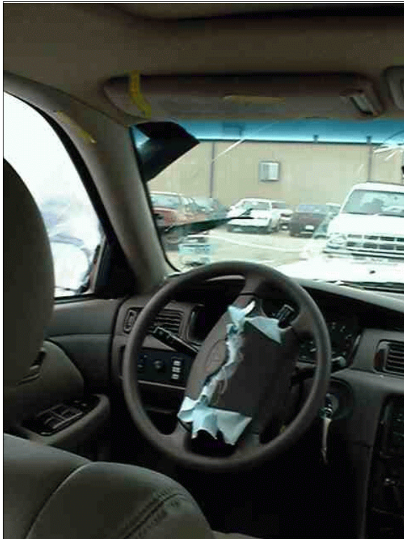
Figure 9: Vertical view of case vehicle's driver seating area showing deployed driver air bag module's cover flaps, remainder of cutout driver's air bag, and probable air bag exhaust gas residue on left "A"-pillar and on left sun visor (case photo #21)
