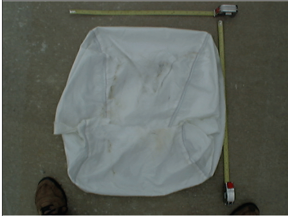
Figure 16: Overhead view of case vehicle's cutout and folded over, front right passenger air bag showing skin evidence on top and underside surfaces (case photo #47)
