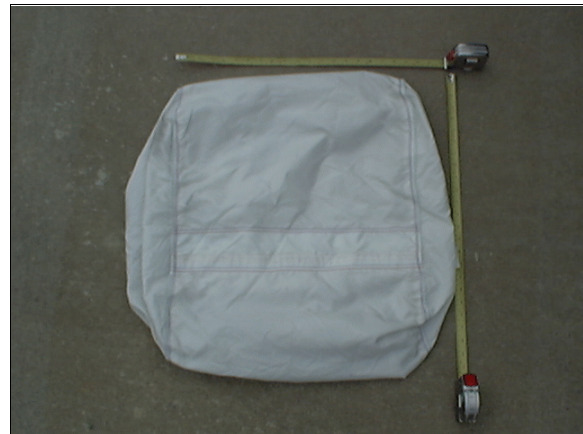
Figure 15: Overhead view of front surface of case vehicle's cutout, front right passenger air bag showing, no visible contact evidence, dimensions, and tether straps (case photo #43)
