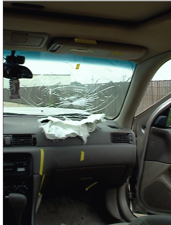
Figure 10: Vertical view of case vehicle's front right seating area showing contacts to instrument panel area (i.e., yellow tape) and sun visor by front right passenger; Note: windshield glazing was cracked by front right module's top cover flap (case photo #32)
