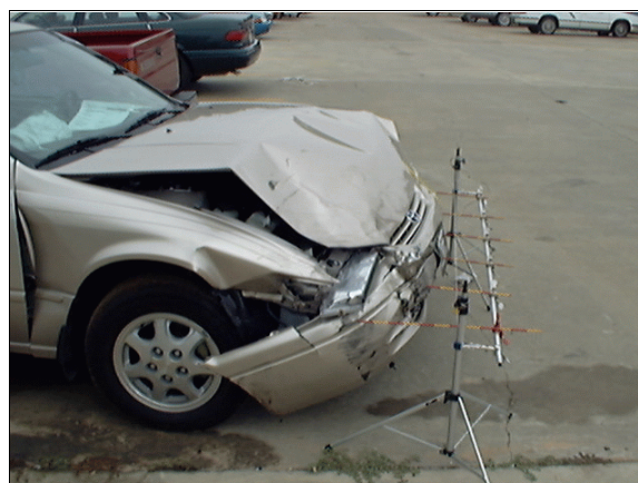
Figure 6: Case vehicle's frontal damage viewed along reference line from right with contour gauge present (case photo #15)
