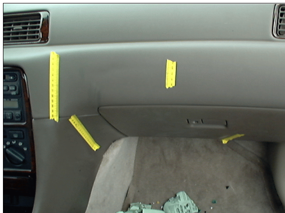
Figure 11: Close-up of contact evidence on case vehicle's center instrument panel and front right knee bolster and glove box door (case photo #34)
