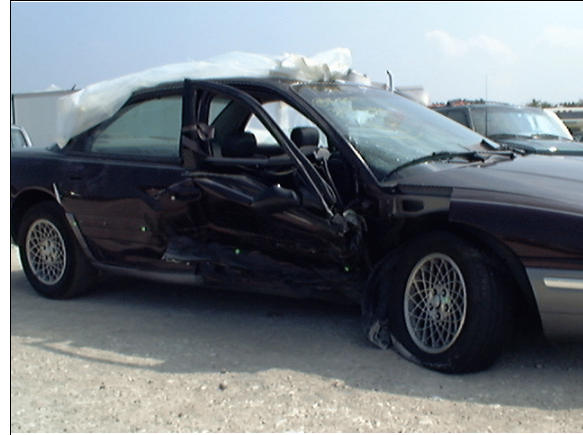
Figure 8: Chrysler's right side damage viewed from front of right (case photo #62)
