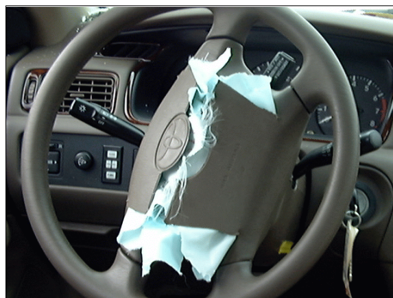
Figure 13: Close-up of case vehicle's steering wheel showing deployed driver air bag module's cover flaps and remainder of cutout driver's air bag (case photo #23)
