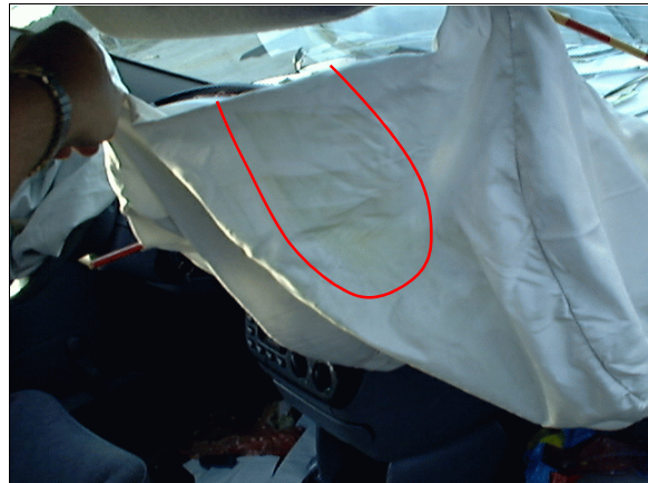
Figure 4: Bottom portion of case vehicle's front right passenger air bag showing green and gold cloth transfers from Green Bay Packers coat passenger was wearing at time of crash (case photo #38)
