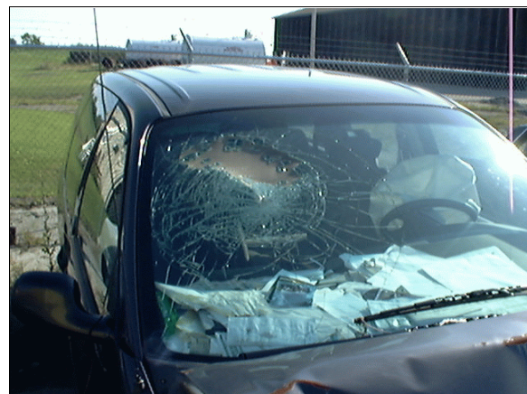
Figure 6: Close-up of case vehicle's windshield contact; Note: the membrane of the deploying air bag was between the passenger's head and the windshield (case photo #19)
