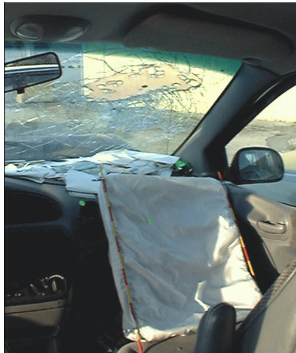
Figure 5: Vertical view of case vehicle's front right passenger seating area; Note: contacts (dots) to dash air vent (broken/scuffed) and front of air bag (skin and cloth transfer) (case photo #35A)
