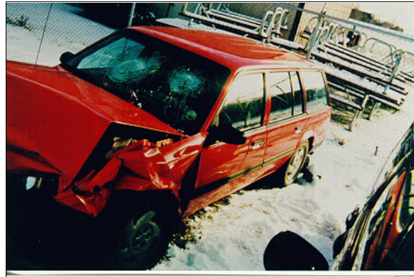
Figure 10: Chevrolet's frontal damage and induced damage viewed from front left while in impound lot (case photo #58)
