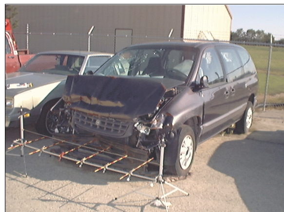
Figure 2: Case vehicle’s frontal deformation viewed from front left with contour gauge present (case photo #10)
