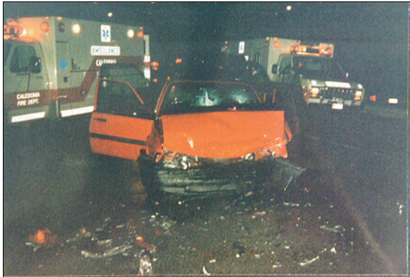
Figure 9: On-scene view of Chevrolet at final rest with both front seat occupants removed; Note: moderate front end damage and head contacts to windshield (case photo #54)
