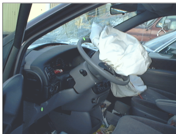
Figure 8: Deformation to upper half of case vehicle's steering wheel rim and contact to knee bolster by driver's left knee (case photo #28)
