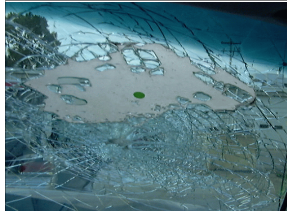
Figure 7: Interior view of contact to case vehicle's windshield from front right passenger (case photo #47)
