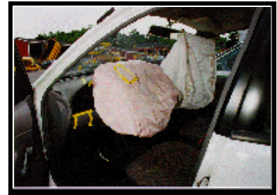
Figure 6. Overall view of the Aspire's deployed frontal air bag system.
