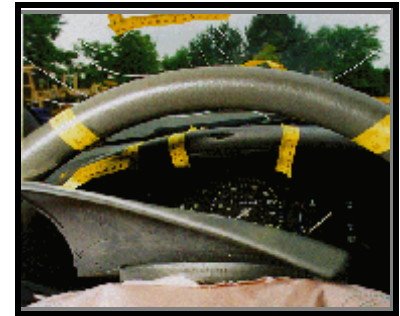
Figure 7. Air bag exhaust gas burn to the upper instrument panel.
