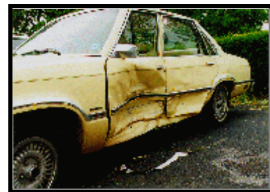
Figure 5. Ford Fairmont's damage pattern.
