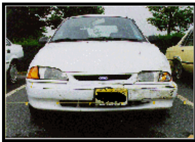
Figure 3. Direct contact damage to the Ford Aspire.
