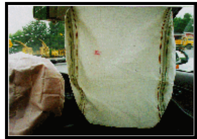
Figure 11. Lipstick transfer to the left side of the passenger air bag.
