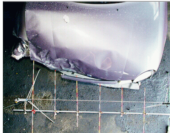
Figure 5: Overhead view of case vehicle's frontal damage/crush measurements (case photo #22)
