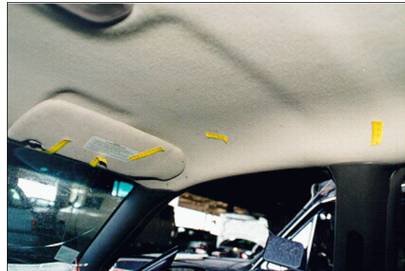
Figure 8: Case vehicle’s front right sun visor and roof showing air bag residue on sun visor and blood splatters on roof from front right passenger (case photo #41)
