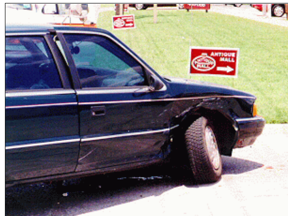
Figure 7: On-scene view of vehicle #2 at final rest; Note: direct damage to right fender and right front wheel assembly (case photo #56)
