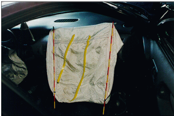
Figure 9: Case vehicle's front right air bag with yellow tape outlining skin transfer to air bag from front right passenger's face (case photo #33)
