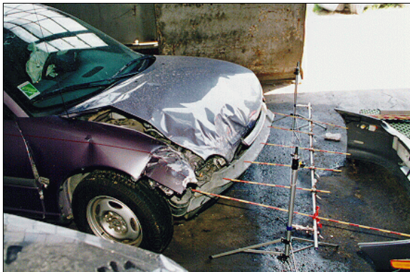
Figure 4: Case vehicle's frontal deformation viewed along reference line from right with contour gauge present; Note: bumper fascia torn away (case photo #18)
