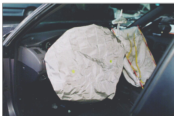
Figure 11: Case vehicle's front seating area showing deployed air bags with contact evidence (i.e., skin transfers) highlighted (case photo #26)
