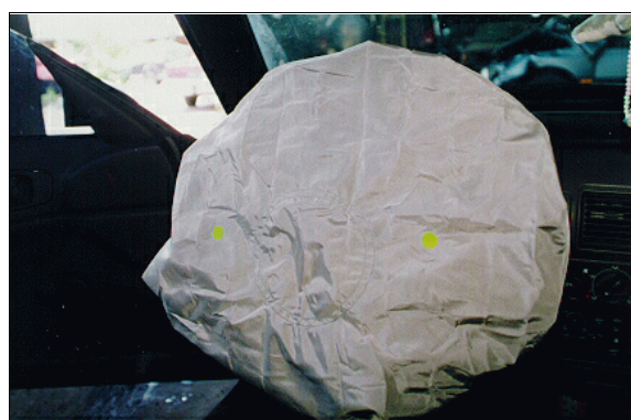
Figure 12: Case vehicle's deployed driver air bag showing contact evidence (i.e., skin transfers); Note: steering wheel inverted 180 degrees (case photo #27)
