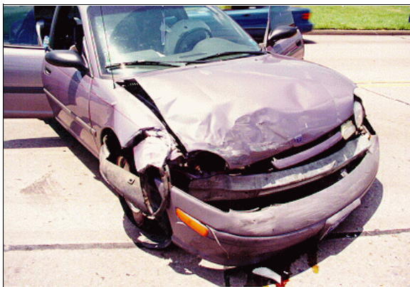
Figure 6: On-scene view of case vehicle at final rest straddling inside northbound lane; Note: frontal damage, particularly to front right (case photo #53)
