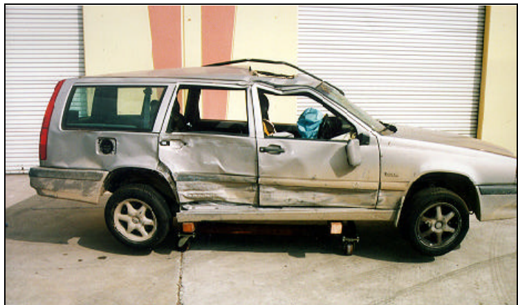
Figure 5. Right side damage to Vehicle 1.
