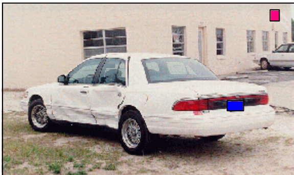
Figure 10: Vehicle #2's left side damage; Note: maximum crush near left rear door handle indicates PDOF acted aft of vehicle's center of gravity (case photo #34)
