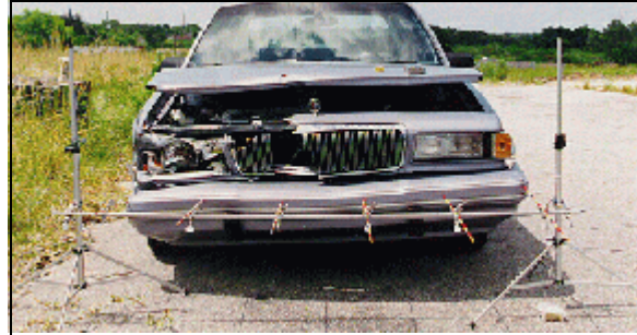
Figure 2: Case vehicle's frontal damage; Note: damage above bumper is primarily to right (case photo #07)
