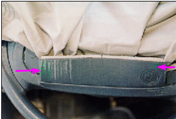
Figure 6: Case vehicle driver air bag module's lower cover flap; Note: green cloth transfer to flap (case photo #22)
