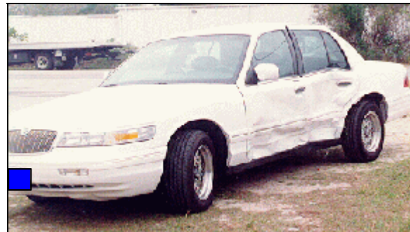
Figure 11: Vehicle #2's left side damage viewed from front showing area of maximum crush near left rear door's handle; Note: since PDOF was aft of vehicle #2's center of gravity, vehicle rotated counterclockwise after impact (case photo #31)
