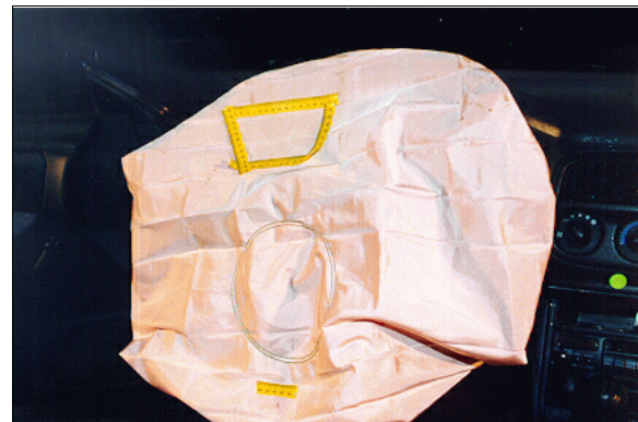
Figure 9: Case vehicle's driver air bag showing contact to upper center front of air bag and blood drops on bottom center (case photo 28)
