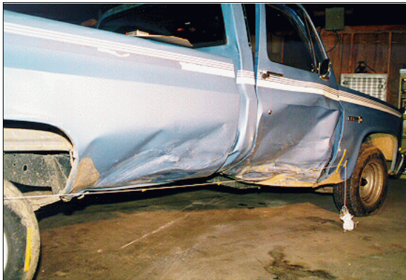
Figure 7: Vehicle #2's damaged right side viewed from back of right (case photo #63)
