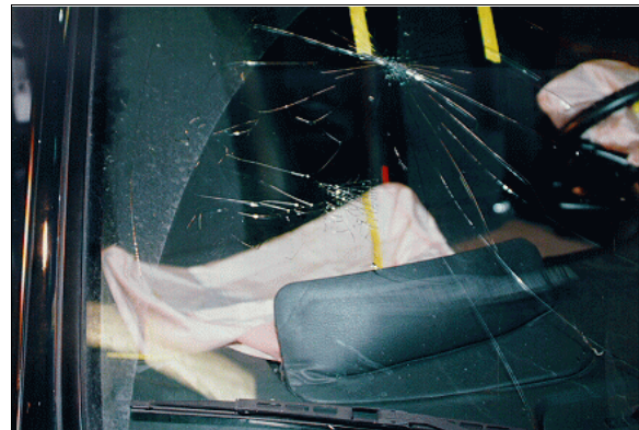
Figure 10: Case vehicle's cracked right windshield and deformed front right air bag module's cover flap (case photo #40)
