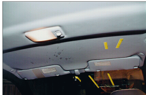
Figure 14: Case vehicle's windshield and roof showing front right passenger's head contact to roof, above front right seat, rearward of header and sun visor (case photo #49)
