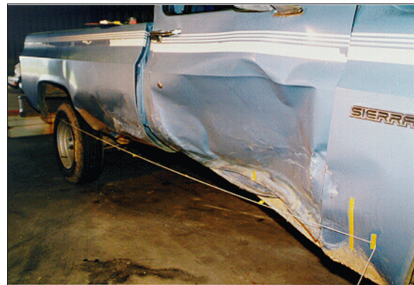
Figure 6: Vehicle #2's right side damage viewed from front of right (case photo #60)
