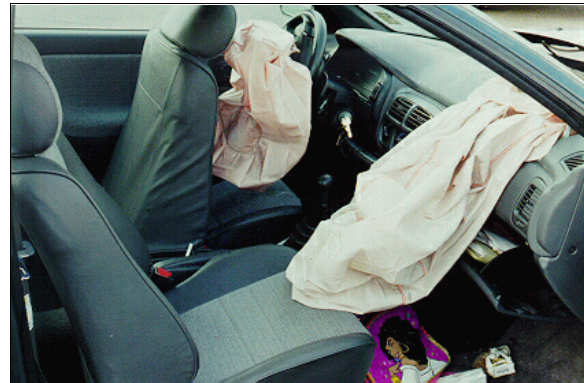
Figure 8: Case vehicle's front seating area showing deployed driver and front right passenger air bags (case photo #15)
