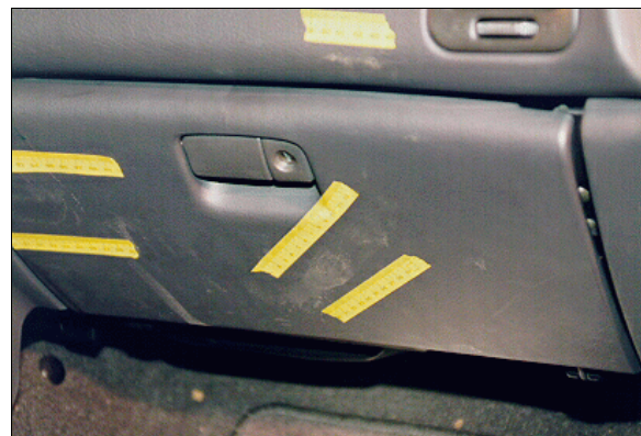
Figure 11: Close-up on contacts on case vehicle's glove box from front right passenger's knees (case photo #46)
