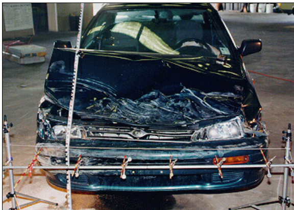
Figure 5: Case vehicle's frontal damage showing rightward shift of left front headlight and hood and hood's under riding interaction with right side of vehicle #2 (case photo #16)
