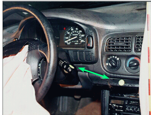
Figure 15: Close-up of contacts to case vehicle's center instrument panel and windshield wiper wand; Note: clump of front right passenger's hair in center instrument panel (case photo #43)
