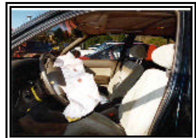
Figure 7. Deployed driver air bag and the vent ports.
