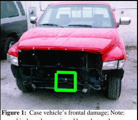
vehi-cle under repair and boxed area shows indentation in bumper reinforcement bar (Case Photo #01)
