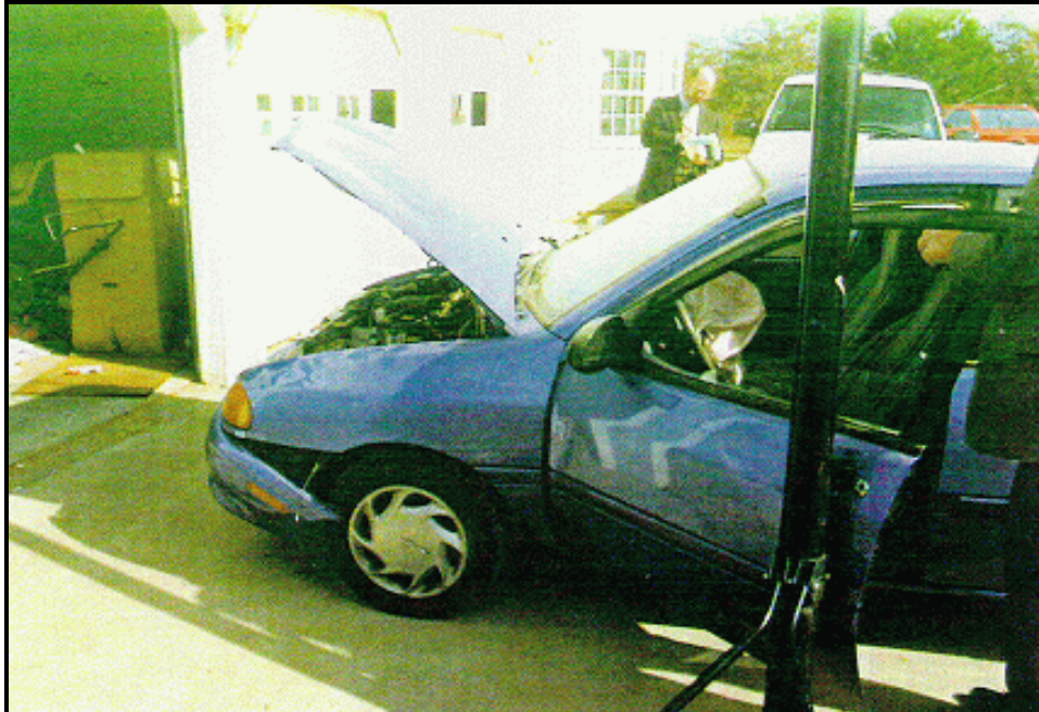
Figure 2: Case vehicle's left side; note: bumper rotated upward (case photo #02)
