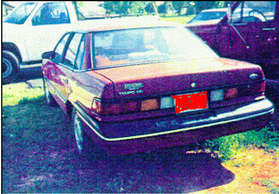
Figure 8: Vehicle #2's back and left side; note: bumper rotated downward (case photo #08)
