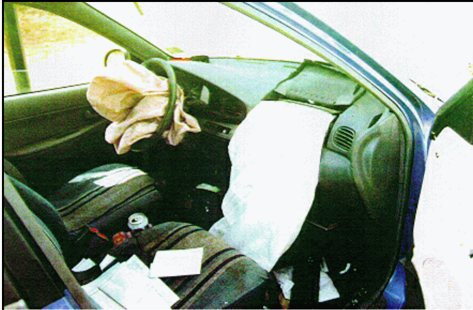
Figure 6: Case vehicle's front seating area; note: driver's seat adjusted near its forward-most position (case photo #06)
