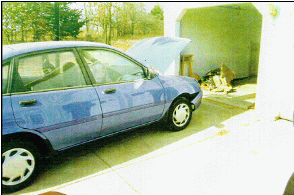
Figure 3: Case vehicle's right side; note: bumper rotated upward (case photo #03)
