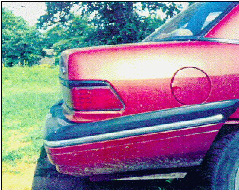
Figure 9: Vehicle #2's right rear corner; note: bumper rotated downward (case photo #09)
