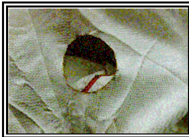
Figure 10. Close-up view of the left vent port of front right passenger air bag
