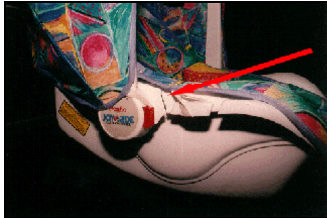
Figure 2. View of cracked infant seat due to instrument panel and air bag contact
