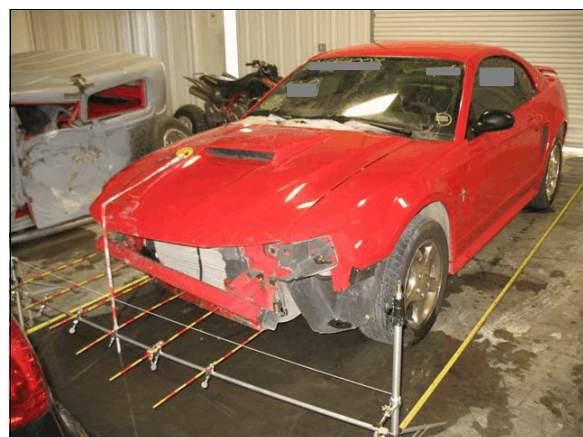
Figure 4: Damage to the front plane of the Ford from the impact to the right side plane of the Hyundai
