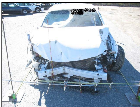
Figure 5: Frontal and oblique damage to the Lexus.
