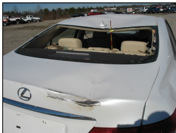
Figure 7: Non-horizontal roof damage to the Lexus.
