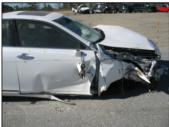
Figure 6: Event 4 sideswipe damage to the Lexus.
