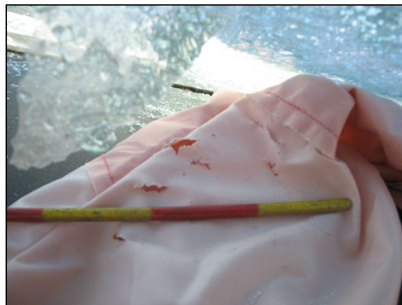
Figure 9: 1-2cm cuts in the upper aspect of the front right air bag, near the windshield.
