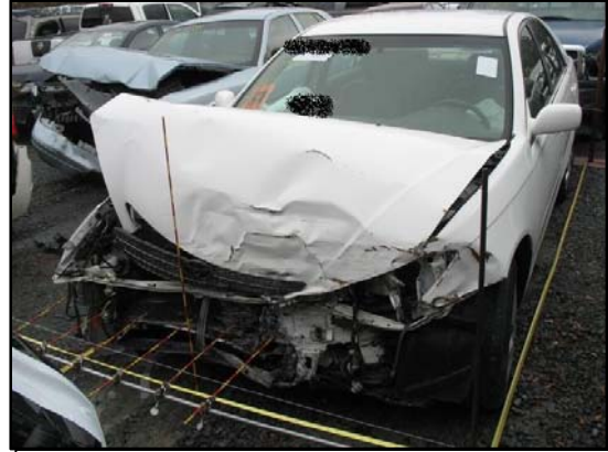
Figure 10: Frontal damage to the Toyota.
