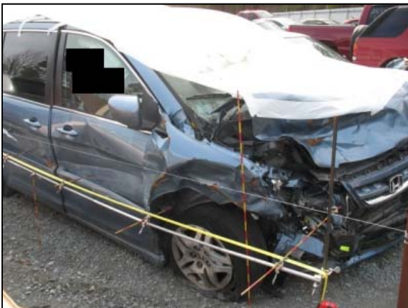
Figure 3: Right plane damage to the Honda resulting from Events 1.
