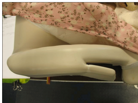
Figure 8: Deformed left belt guide on second row right CRS
