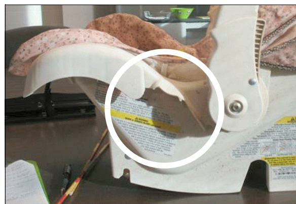
Figure 5: Second row left CRS with damaged left flange
