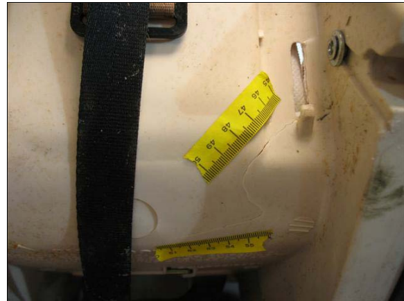
Figure 6: Cracked bottom of second row left CRS
