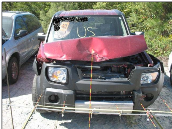
Figure 8: View of the frontal damage to the Honda.
