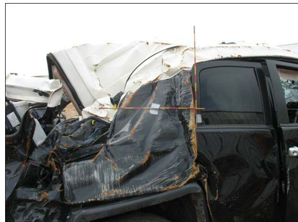
Figure 6: Max vertical crush to right rear roof area
