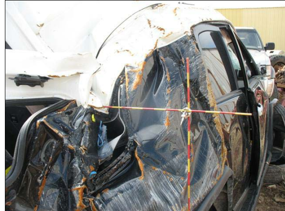
Figure 5: Lateral max crush on right roof rail
