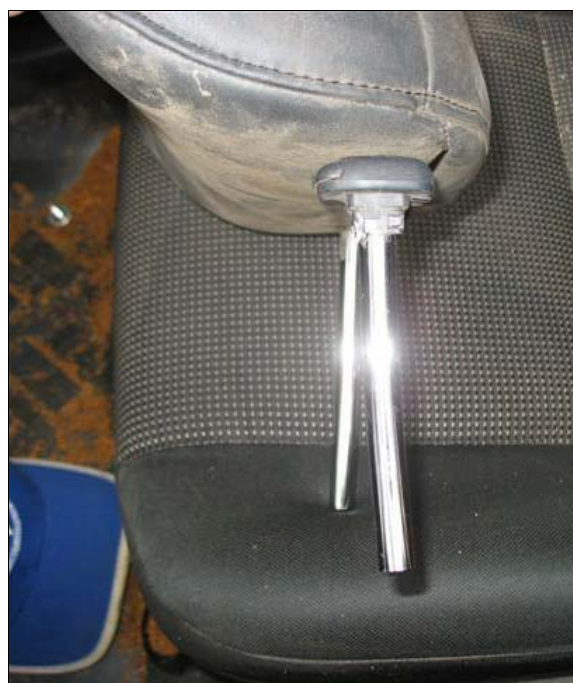
Figure 8: Driver's deformed head restraint posts
