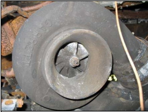
Figure 12. Intake impeller and cast alloy housing of the turbocharger.
