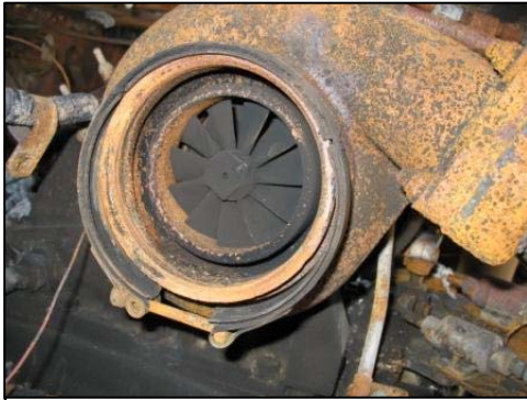
Figure 14. Exhaust impeller and cast iron housing of the turbocharger.
