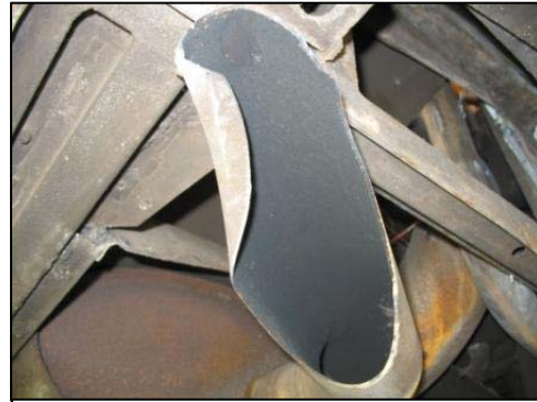
Figure 15. Carbon deposits in the tailpipe of the motorcoach.
