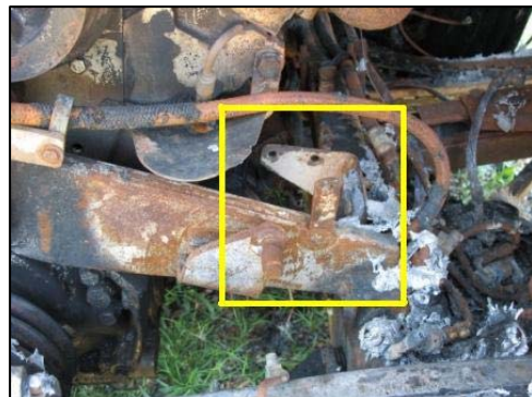
Figure 19. Presumed mounting points of the alternator.
