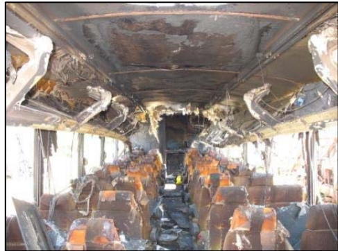
Figure 10. Rear interior view of the fire damage to the interior of the motorcoach.
