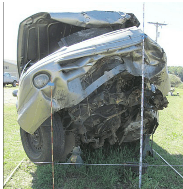
Figure 6: Damage on the front plane and undercarriage of the Dodge from the impact with the 130 cm (51.2 in) tree; scale on right in 10 th s of meter; each increment on left scale is 5 cm (2 in)
