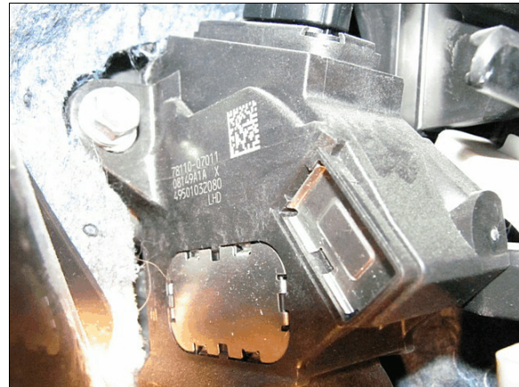
Figure 8: The CTS accelerator mechanism housing
