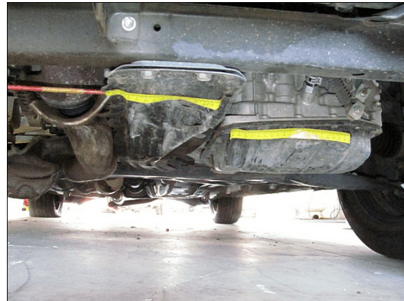
Figure 3: Yellow tape and colored rod show area of damage on the front undercarriage and bottom of the engine
