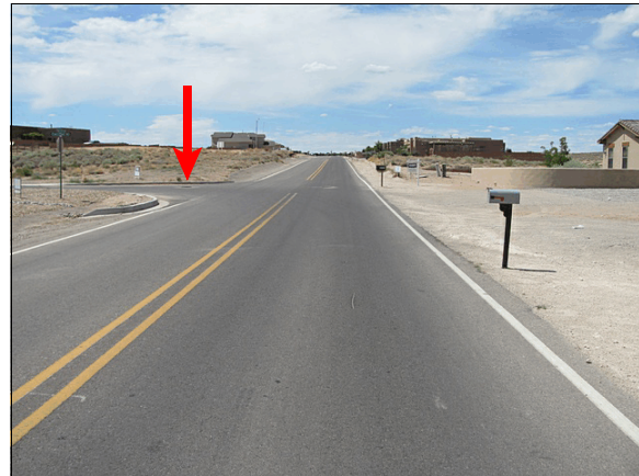
Figure 2: Approach of the Toyota to the intersection; arrow shows location of impact with 20 cm (7.9 in) high concrete curb
