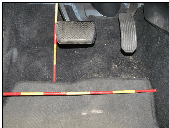
Figure 6: The initial status of the brake pedal, accelerator pedal, and Toyota floor mat at the SCI inspection; please note that the vertical scale does not represent the centerline of the driver's seat
