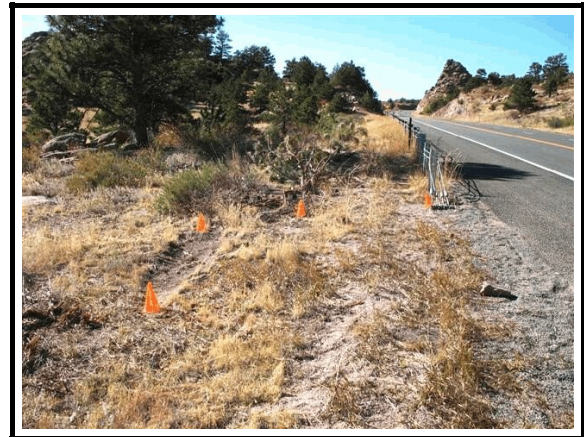
Figure 3. Crash site showing locations of tire furrow (left), tree impact (center) and cable rail barrier impact (right)
