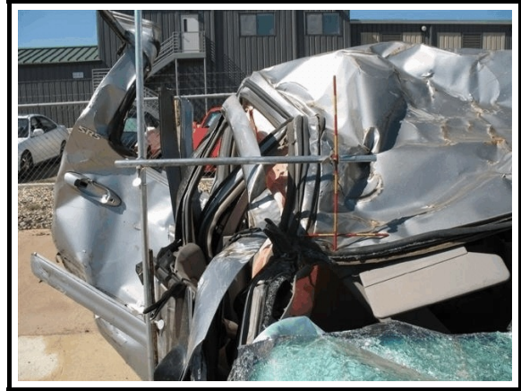
Figure 4. Maximum vertical crush to greenhouse documentation
