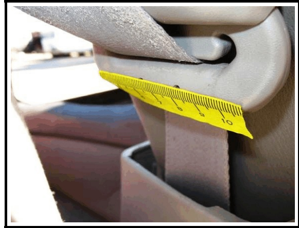
Figure 5. Front right occupant's safety belt webbing and D-ring showing evidence of loading
